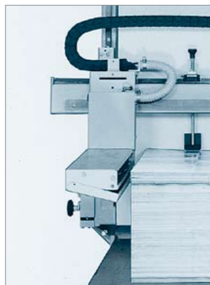
Stapelheber Profi-Line PH 1-BF with bilateral air blast
